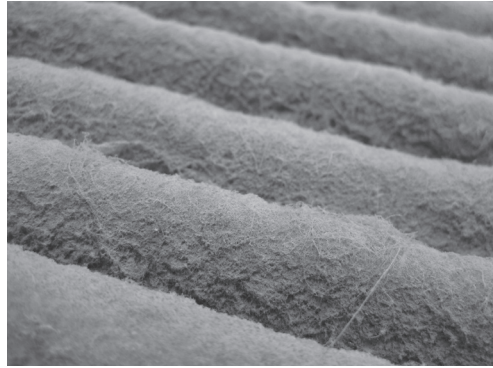
Pleated air filters perform better than flat ones.
