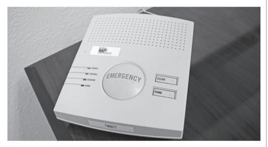
NAEC's Personal Emergency Response System includes a console with a large emergency button as well as a waterproof wireless transmitter that can be worn as a necklace or wristband.
